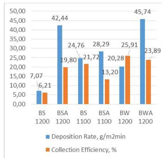
**Figure 12:** Ash deposition rate and collection efficiencies for temperature of experiments: 1100°C and 1200°C (USTUTT).
