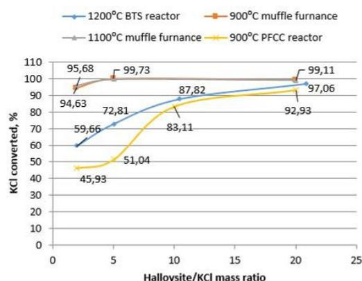
**Figure 5:** KCl converted in different temperature and process conditions.
