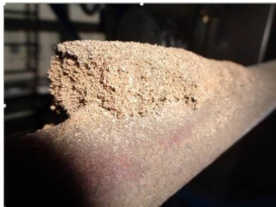
**Figure 10:** Ash deposit collected during DS4 900°C tests - close-up image, powdery deposit; PFCC reactor.
