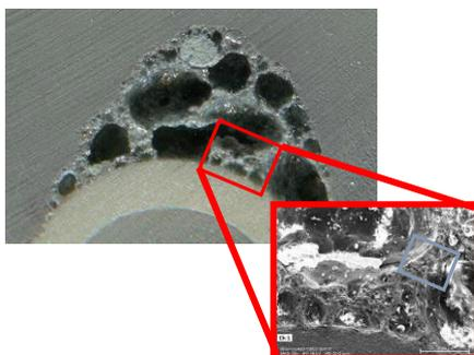
**Figure 13:** Microscopic picture and secondary electron image (SE) of the selected cut and area of the BS 1100 deposit sample for the SEM-EDX analysis
