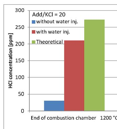
**Figure 6:** Measured and theoretical HCl conc. for halloysite/KCl=20.
