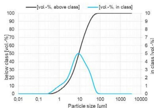
**Figure 1:** Particle size distribution of the used halloysite (USTUTT).
