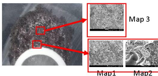
**Figure 15:** Microscopic picture and secondary electron images (SE) of the selected cut and areas of the BSA 1100 deposit sample for the SEM-EDX analysis.
