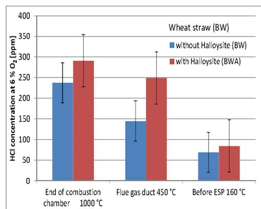
**Figure 7:** Measured HCl con. during combustion of wheat straw with (BWA) and without additive (BW).
