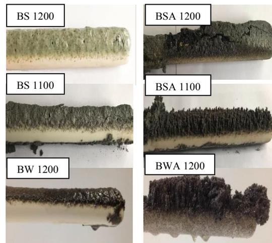
**Figure 11:** Pictures of the ash deposits collected on the ceramic probes during the BTS tests.
