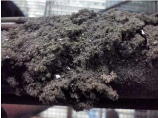
**Figure 9:** Ash deposit collected during DS0 900°C tests - close-up image, visible sintered ashes and agglomerates; PFCC reactor.
