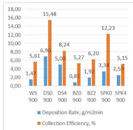
**Figure 8:** Ash deposition rate and collection efficiencies for temperature of experiments: 900°C (SUT).
