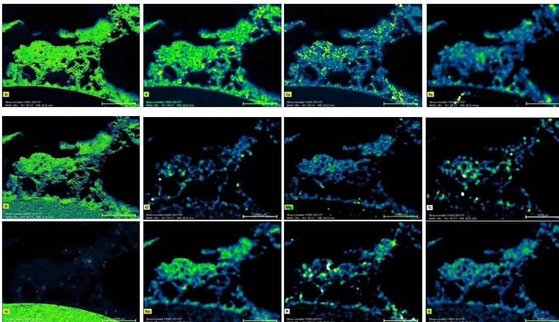
**Figure 14:** SEM-EDX mapping of the selected area of the BS 1100 deposit sample.
