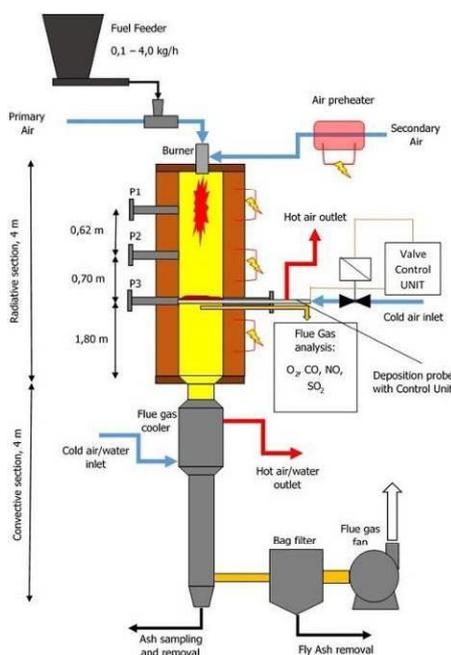
**Figure 3:** Pulverized Fuel Combustion Chamber located in the IPET (SUT).
